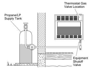
Figure 23 - Checking Gas Joints
